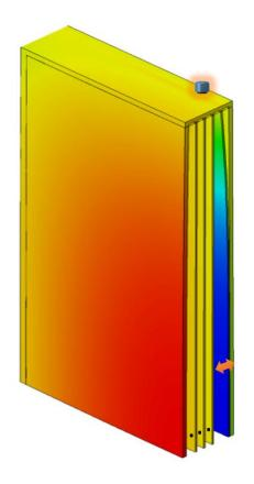
Q-Air is commonly equipped with a dedicated, flexing expansion glass and a breathable innermost chamber. In this way, climatic stress to the unit is reduced.
