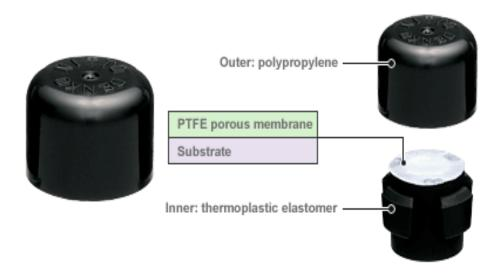
Q-Air breather is carry-over technology from the automotive headlamp industry where it is in use for 20 years on millions of units sold. Its purpose is to prevent entry of liquids through the pressure equalization pathways.
