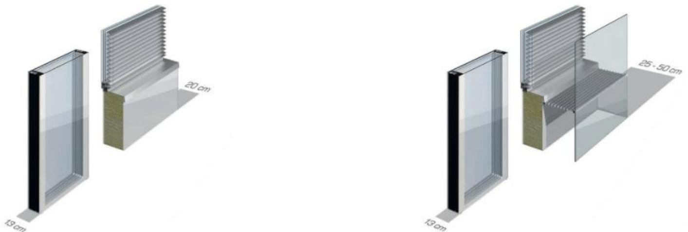
Q-Air facades are usually less than 15 cm thick. Conventional solutions with comparable performance such as triple-pane glazing with parapets could easily reach 40 cm thickness of mineral wool insulation. In such cases, Q-Air façade saves 20-25 cm space. In some cases, this is sufficient to pay-back the extra investment cost into the Q-Air<sup>4</sup>.
