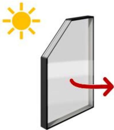
Experience teaches us that sitting behind the glass in the sunny summer day might bring discomfort from radiating heat. This phenomenon becomes apparent when the nominal calculated glass solar gain (g-value) exceeds 0.3. Basic glass units might pour heat inward through pure conduction.
