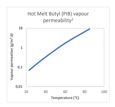
PIB primary seal increases vapour permeability with the temperature a lot (left image)<sup>3</sup>; more than a hundred-fold from room temperature to 80°C. It is of paramount importance for the multipane glass unit longevity to always keep middle glass pane's temperatures at below of 70°C. This keeps PIB permeability at less than 1.5 g/m<sup>2</sup>d which is upper design value for the insulating glass<sup>4</sup>.
