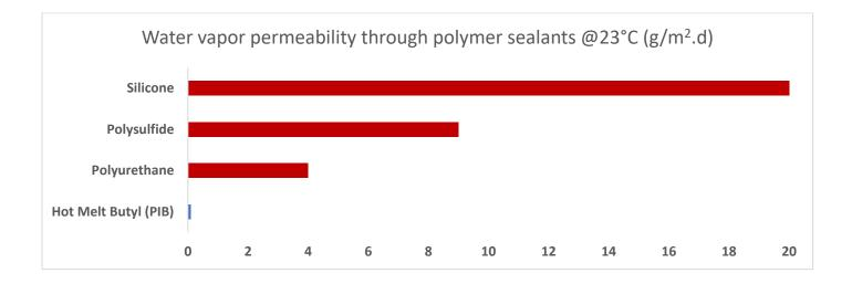
Purpose of the secondary seal (silicone, polysulfide, polyurethane) is to hold the primary seal in place<sup>2</sup>. Increased summer insulating gas pressure, spacer to glass length variations will stretch the primary PIB seal and thus reduce its effectiveness as water vapour barrier. Viscoelastic mechanical properties of secondary seal play an essential role in assuring the long-lasting effect of Low-E coatings<sup>2</sup>.
