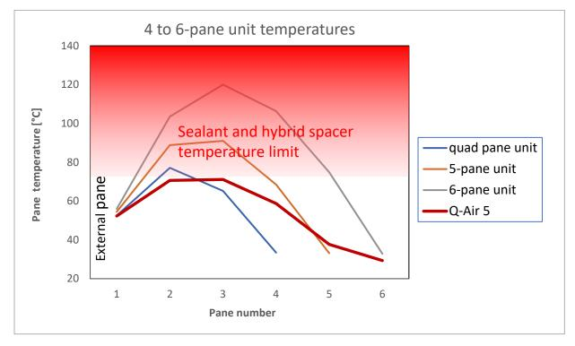
In the diagram above temperatures of individual glass panes in contact with the primary seal are shown for various unsophisticated multipane glass arrangements and the Q-Air as reference.
